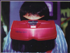
The VB is too heavy to strap onto your head, so it sits on a minitripod.
