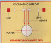
(ABOVE) The 3-D graphics are created by reflecting four shades of red on a black background off oscillating mirrors. The minute vibrations of the mirrors give the image its virtual thickness and density.
